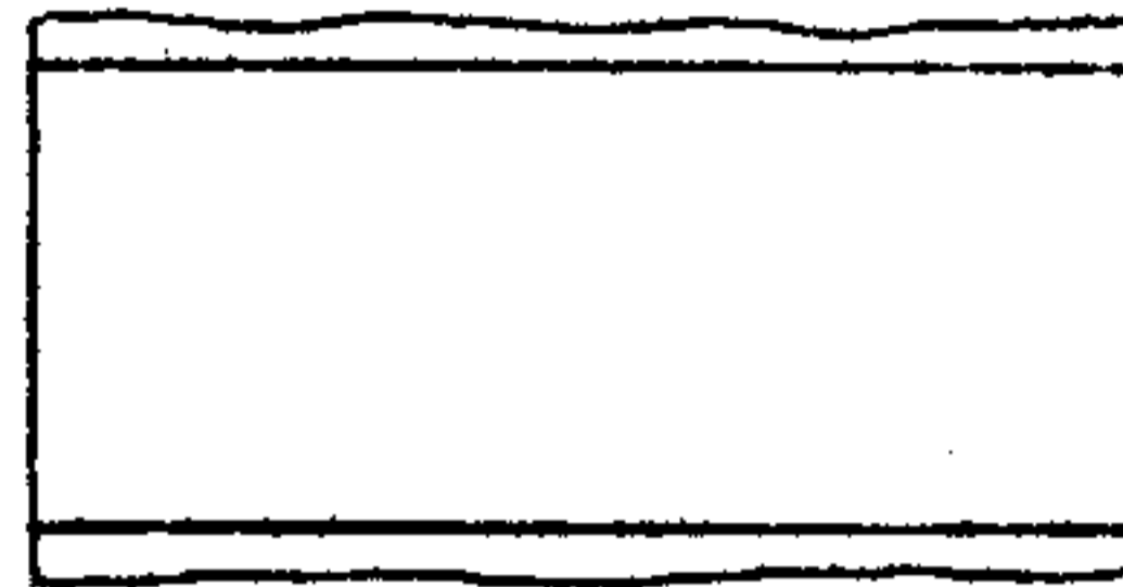
GOOD SSB SIGNAL, TONE INPUT WITH SMALL PER- CENT OF SPURIOUS RADIA- TION (RF)
